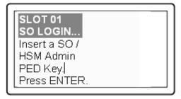
Authenticate as Security Officer by supplying the appropriate HSM SO PED Key that was imprinted during the HSM initialization step. The PED might prompt you for the numeric password PED PIN that might optionally have been assigned to the HSM SO PED Key. Luna PED provides the HSM SO authentication secret to the Luna HSM.
